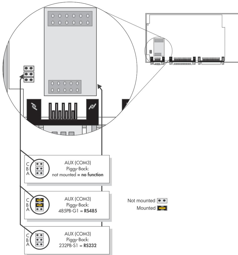
**Fig. 7.3:** Jumper configurations for the “AUX (COM3)” port (internal)
