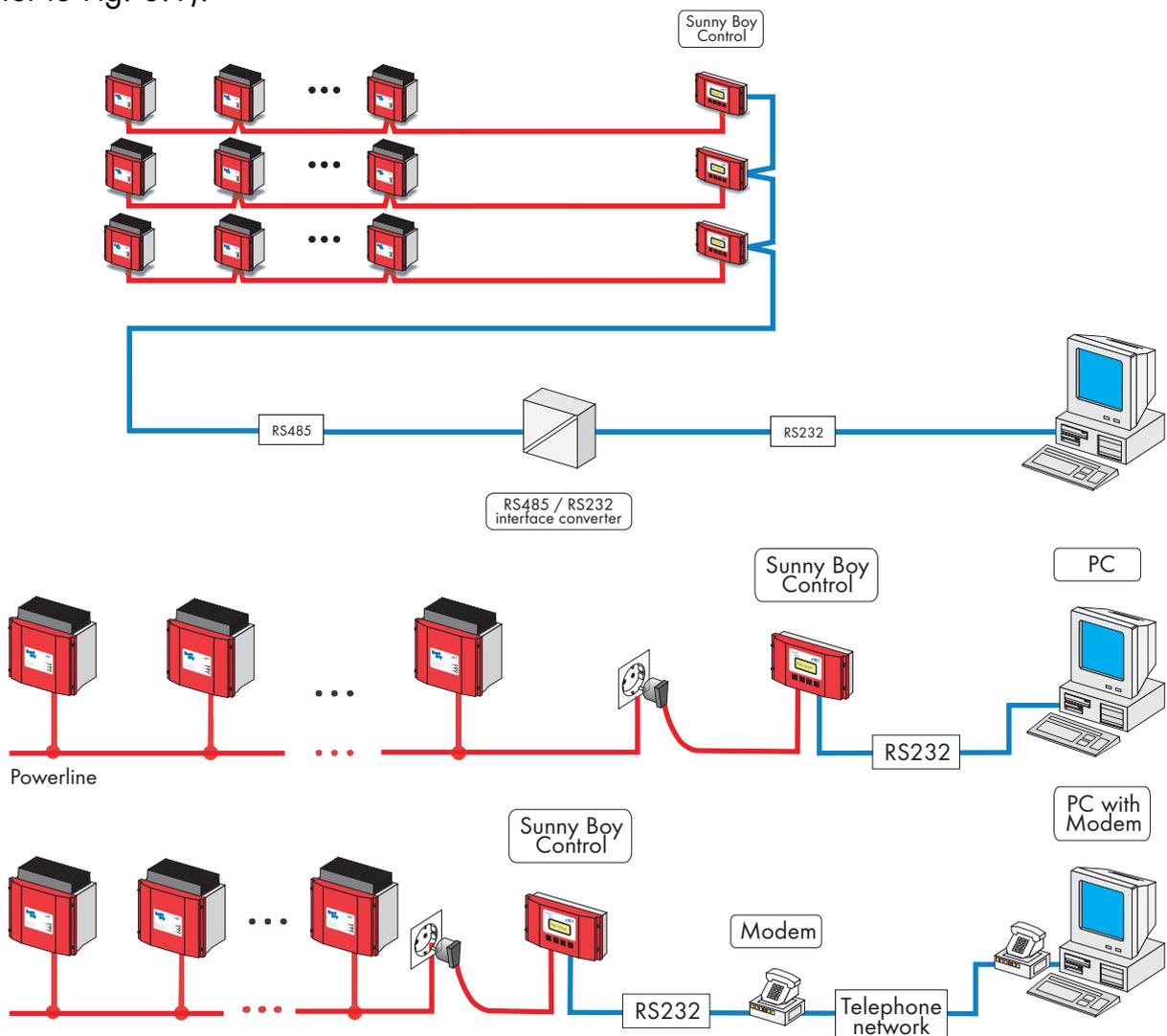
**Fig. 8.1:** Various configurations using a PC and Sunny Data Control
