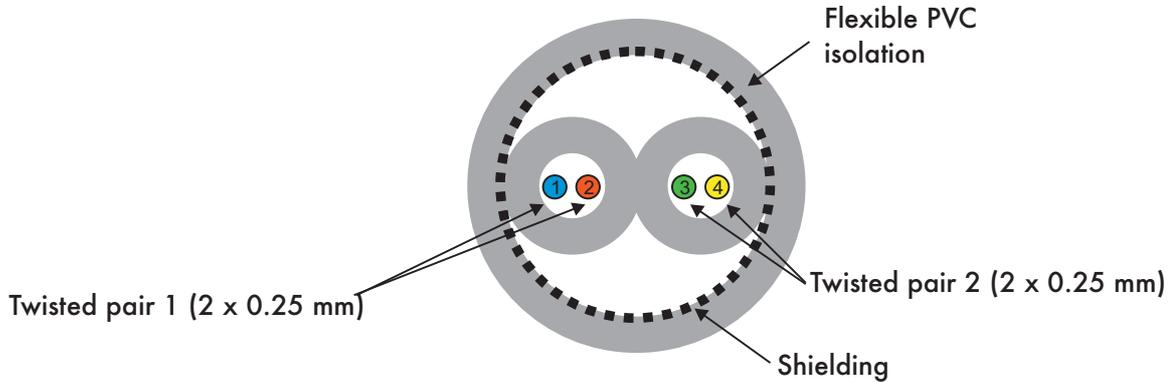
**Fig. 3.6:** Recommended cable for RS485 communication
