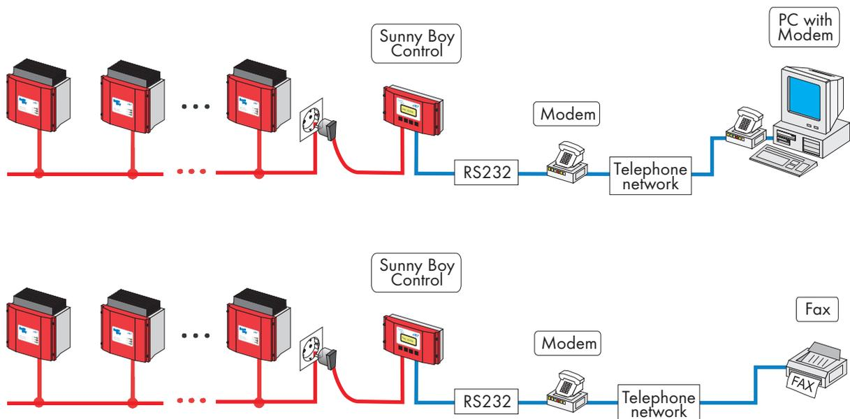
**Fig. 3.17:** Modem connection for remote access (top) and fax transmission (bottom)
