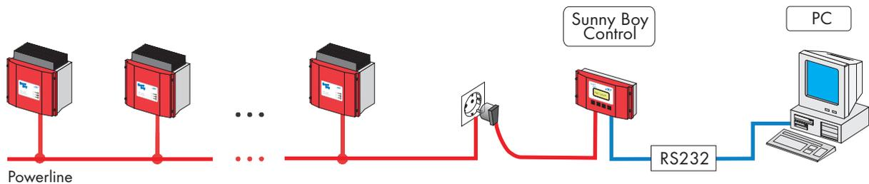
**Fig. 3.10:** RS232 connection to a PC
