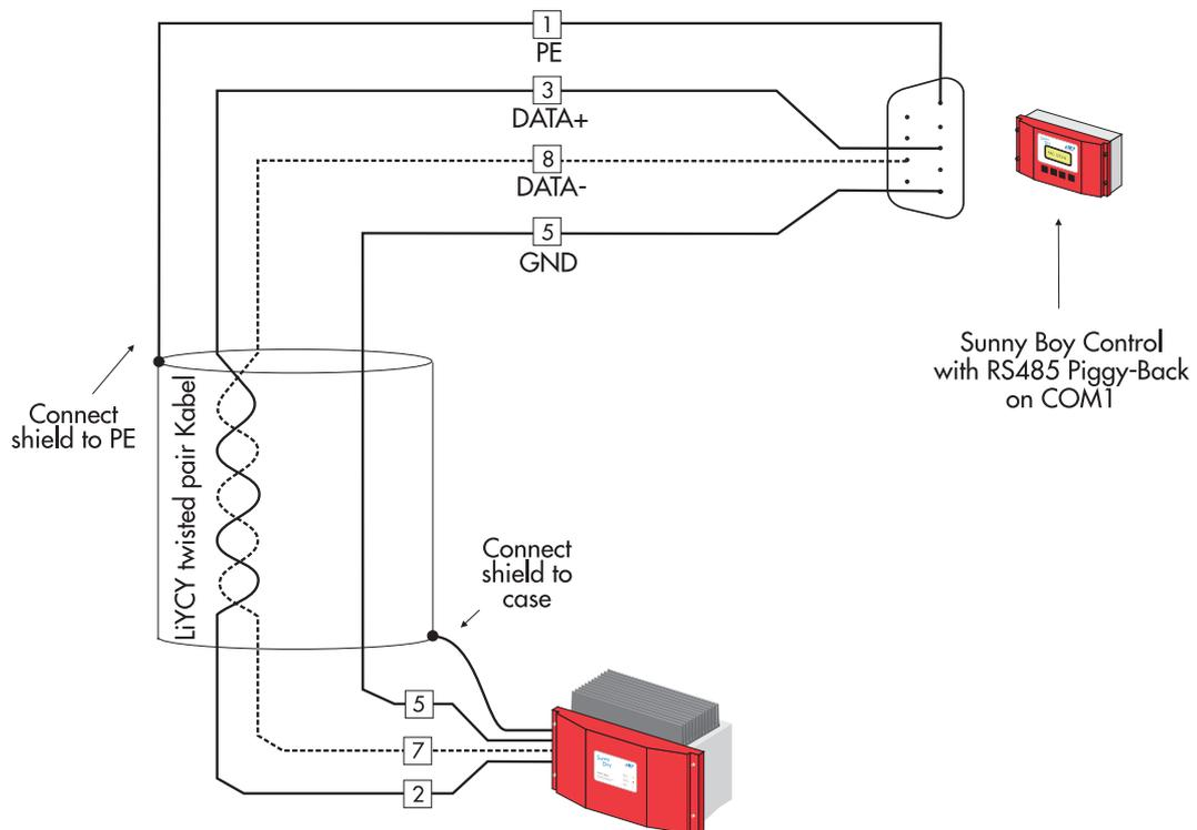
**Fig. 3.7:** RS485 connection between one Sunny Boy and a Sunny Boy Control
