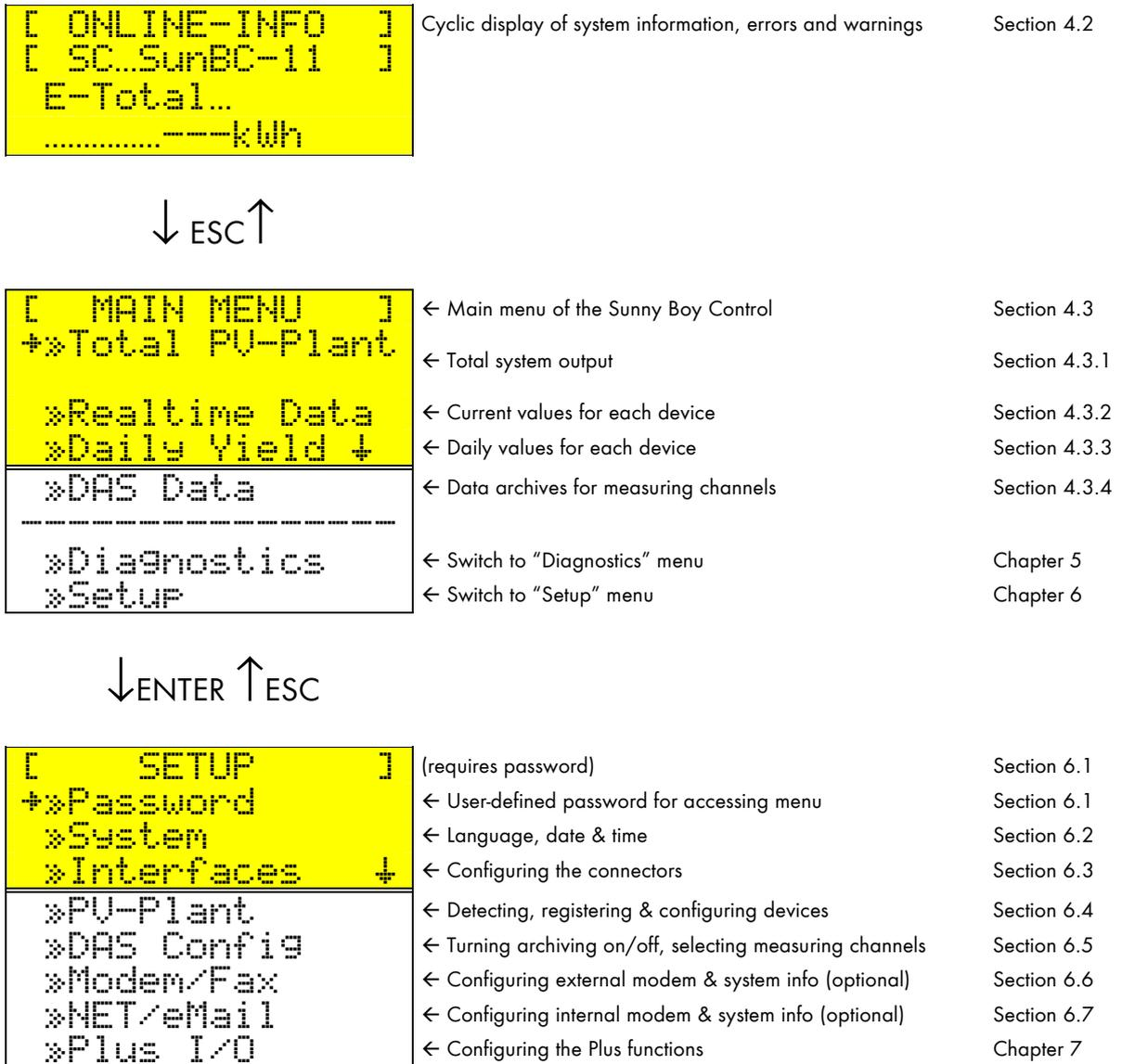
**Fig. 4.2:** Menu structure of the Sunny Boy Control
