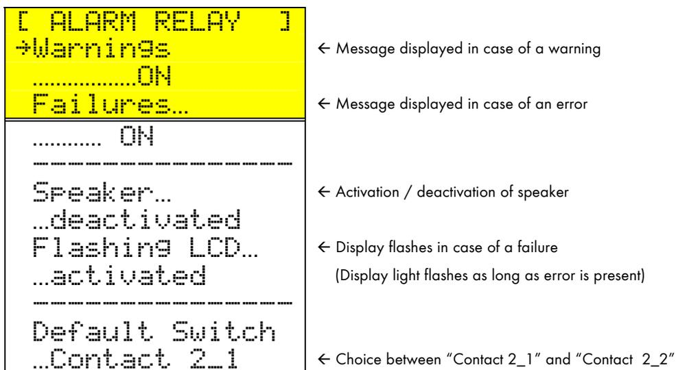
**Fig. 6.12:** Alarm contact screen
