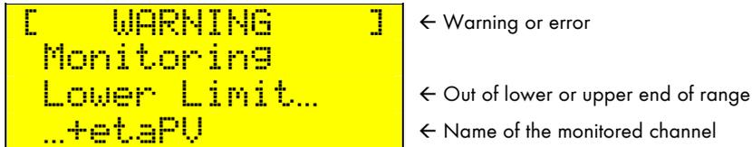
**Fig. 9.7:** Example of monitoring warning
