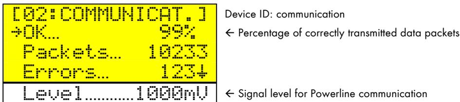
**Fig. 9.14:** Communication test
