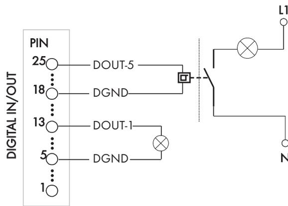
**Fig. 7.18:** Digital output channel application
