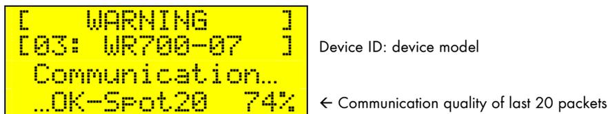
**Fig. 9.2:** Example of communication warning
