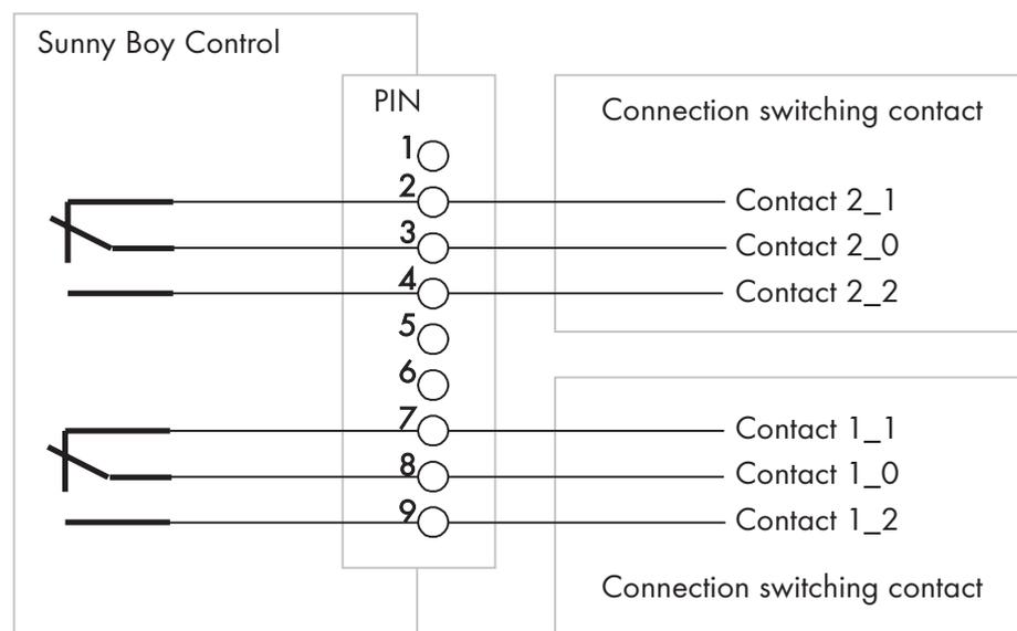
**Fig. 3.18:** Diagram of "Relay Out" connector
