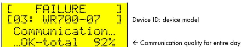
**Fig. 9.4:** Example of communication failure
