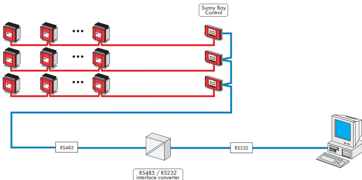
**Fig. 3.15:** RS485 connection between a PC and several Sunny Boy Controls
