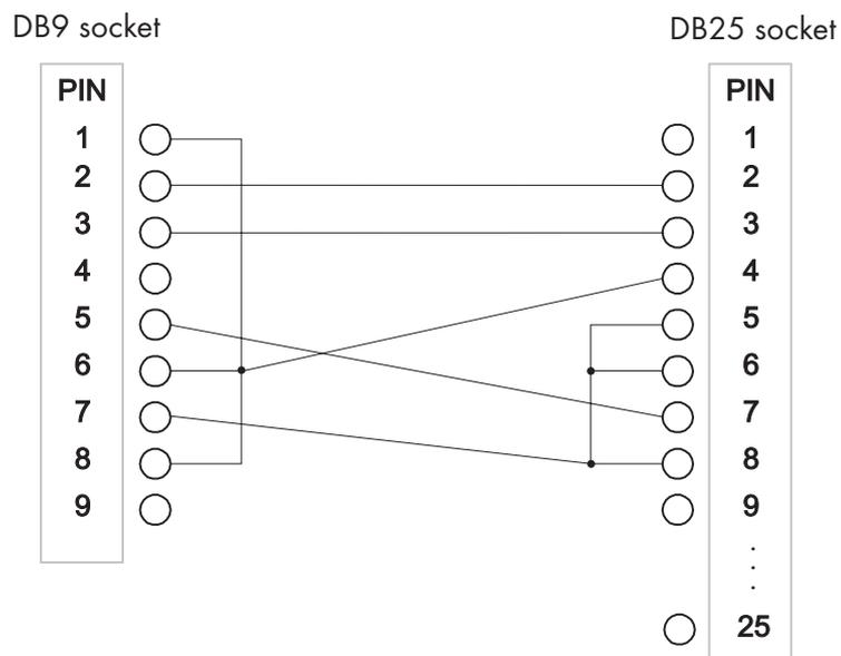
**Fig. 3.12:** Diagram of DB9-DB25 cable for PC connection
