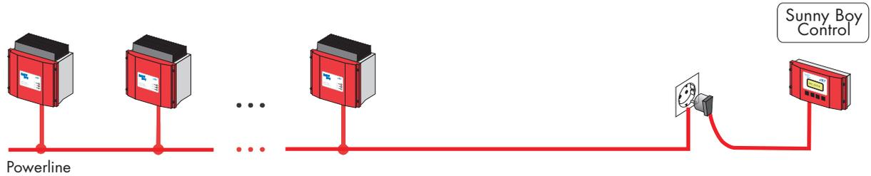
**Fig. 3.3:** Powerline communication
