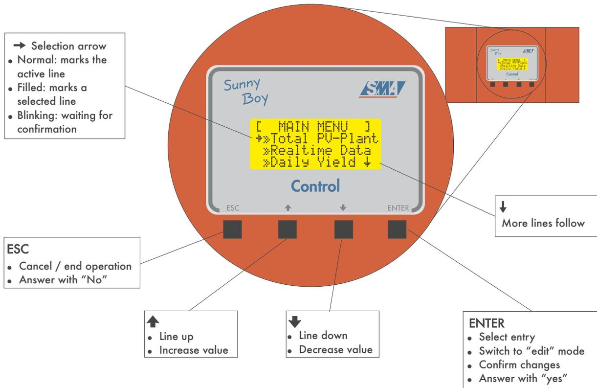
**Fig. 1.1:** Operation panel of the Sunny Boy Control
