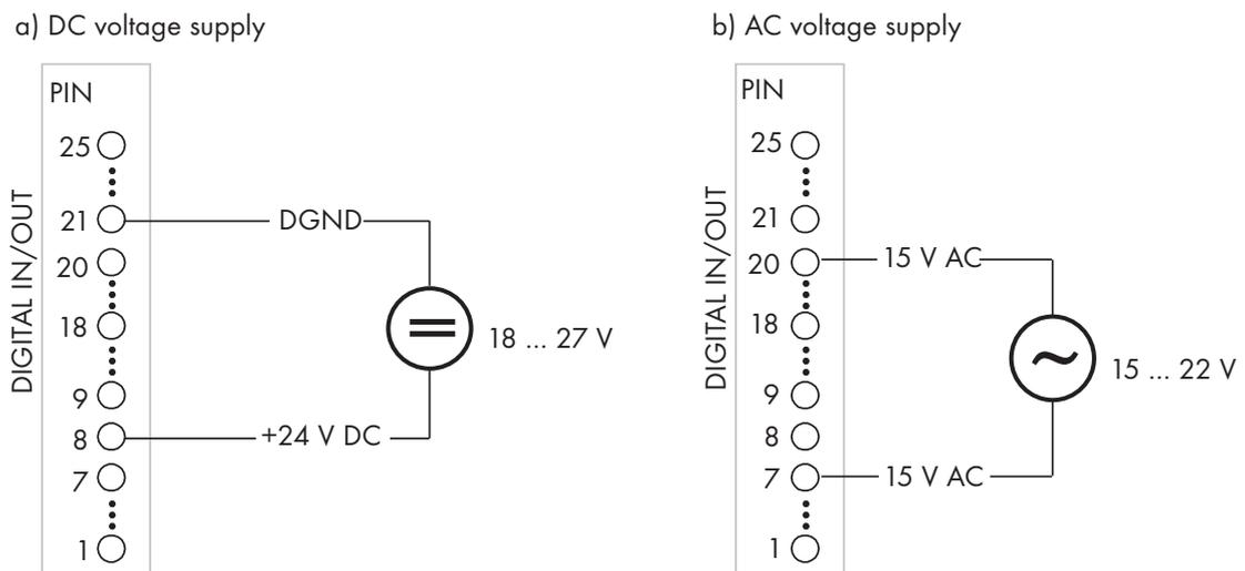
**Fig. 7.14:** Supplying power to the digital interface (example)
