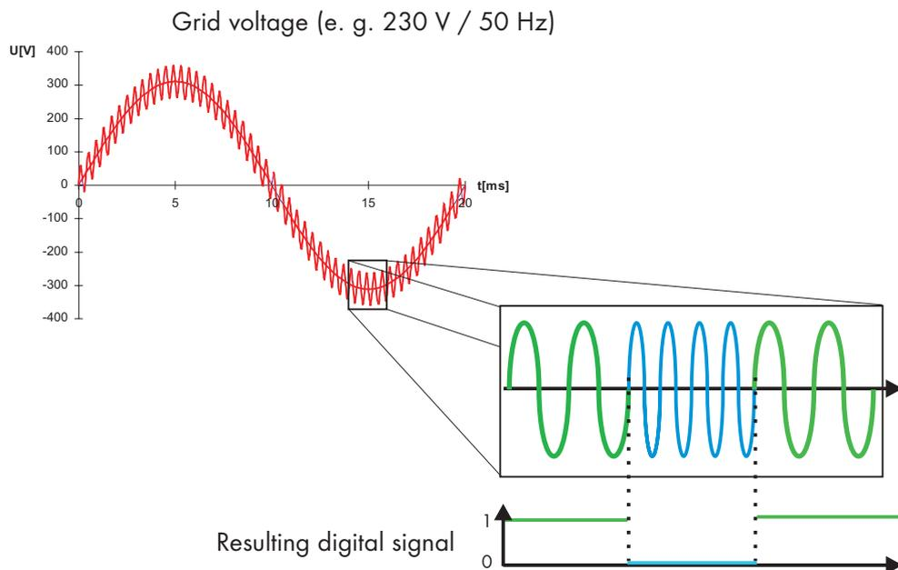
**Fig. 9.8:** Principle of Powerline communication
