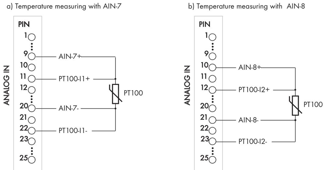
**Fig. 7.10:** Connections for temperature input channels AIN-7 and AIN-8
