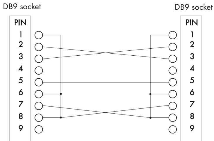
**Fig. 3.11:** Diagram of DB9-DB9 cable for PC connection
