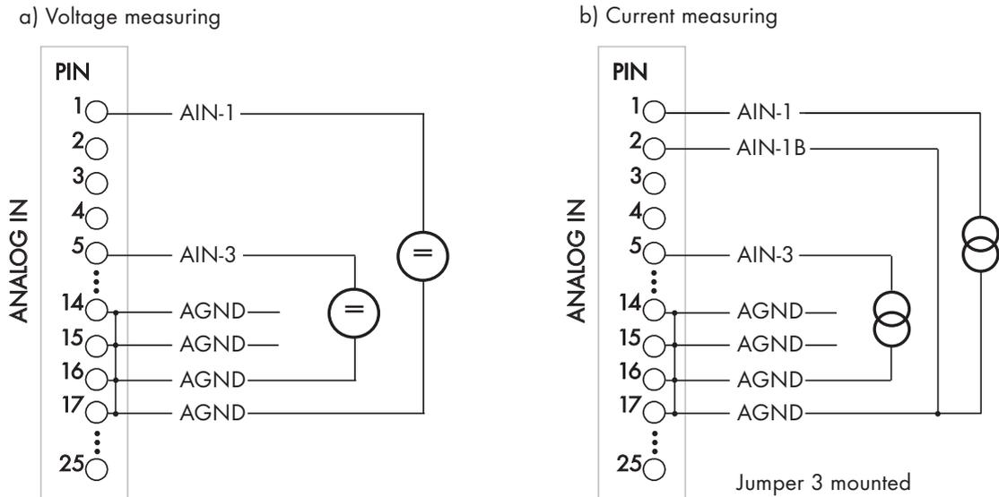
**Fig. 7.5:** Analog input connection examples
