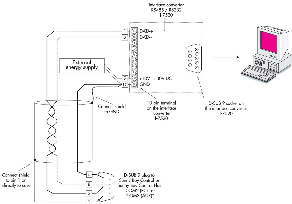
**Fig. 3.14:** RS485 connection between a PC and a Sunny Boy Control
