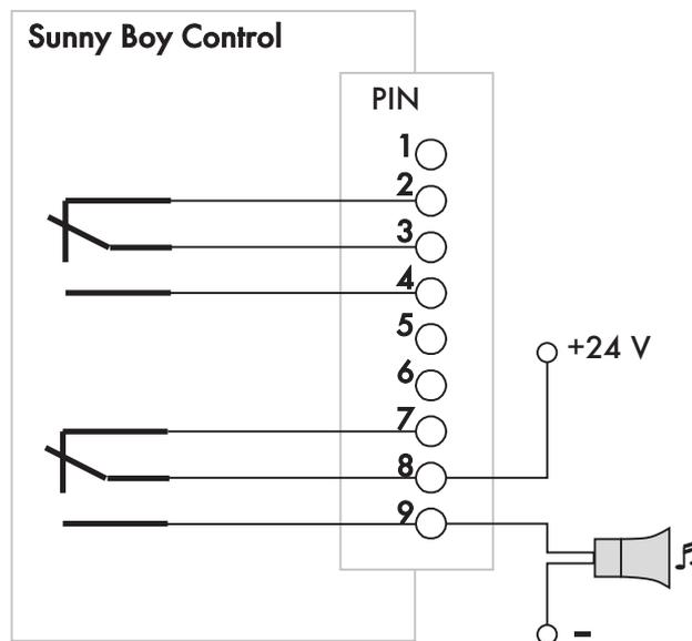
**Fig. 3.19:** Alarm contact application
