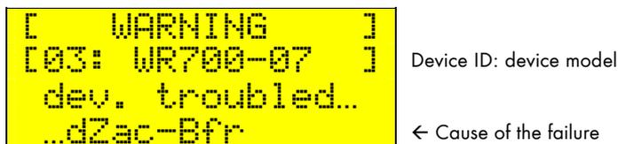
**Fig. 9.1:** Example of device failure
