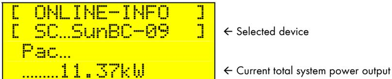
**Fig. 4.3:** Current total system power output in Online-Info
