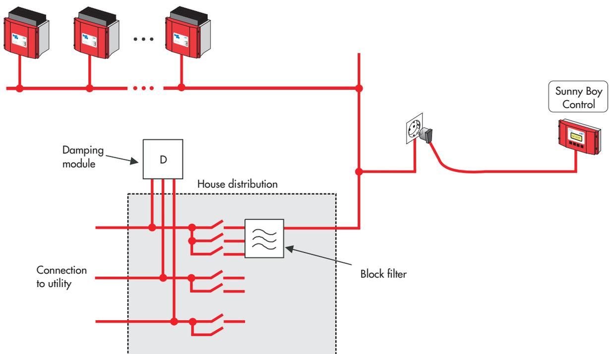
**Fig. 9.11:** Interference suppression in case of strong noise
