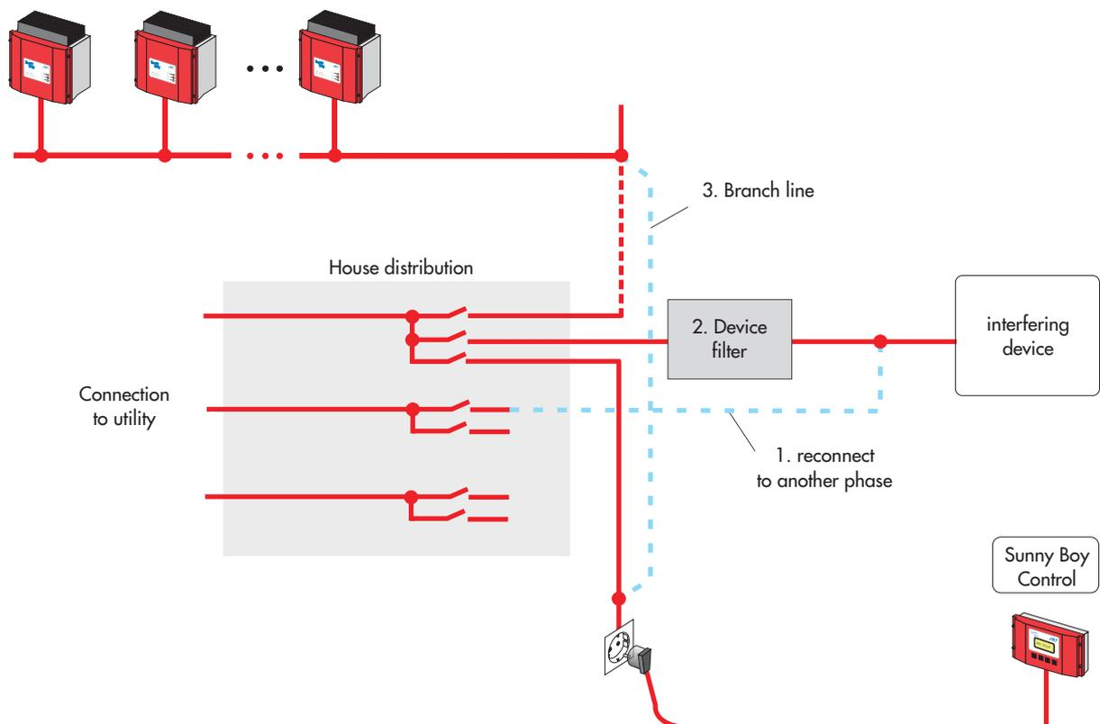
**Fig. 9.9:** Interference suppression in case of strong signal damping
