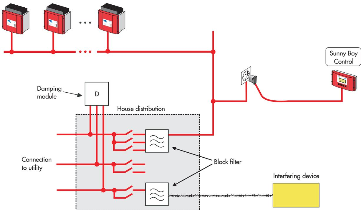
**Fig. 9.12:** Suppressing interference from multiple communication systems
