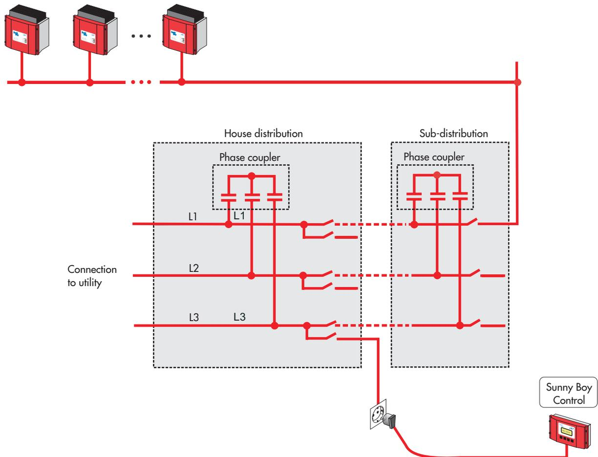
**Fig. 9.10:** Interference suppression in case of phase coupling
