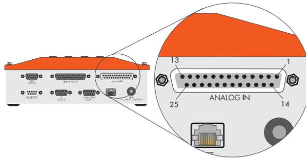
**Fig. 7.4:** “ANALOG IN” connector
