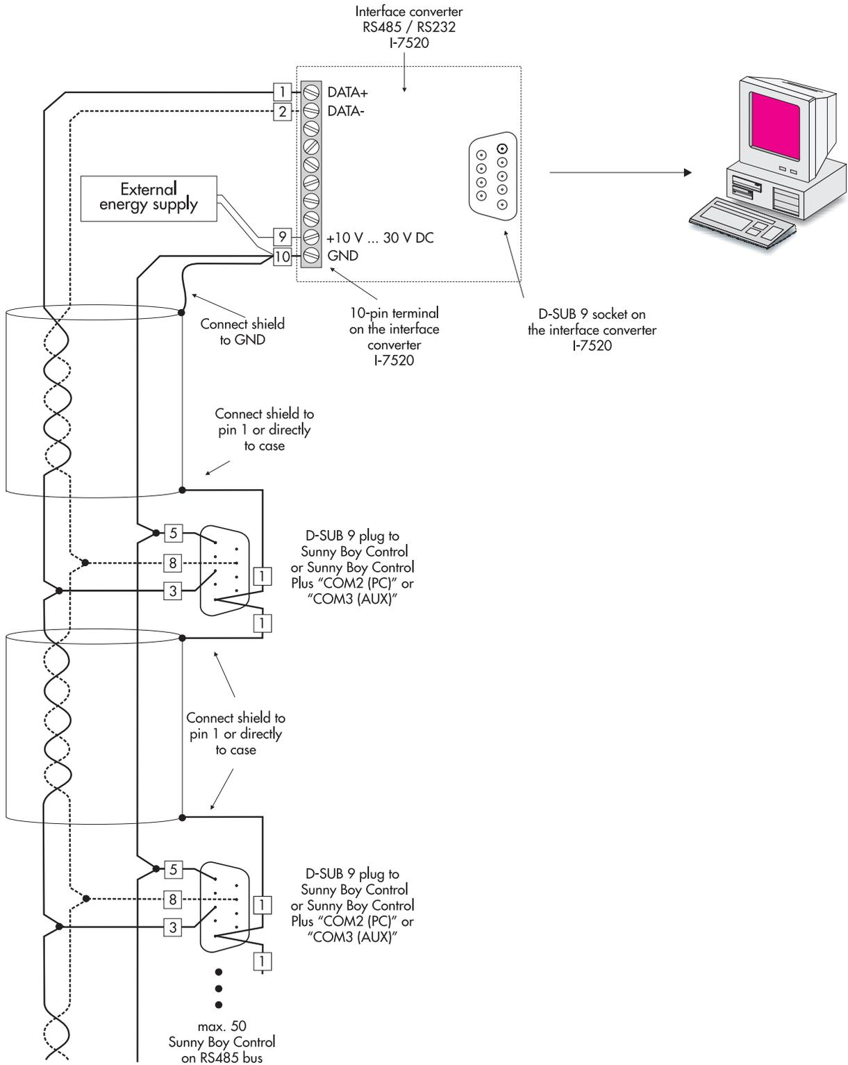
**Fig. 3.16:** Connection between a PC and several Sunny Boy Controls
