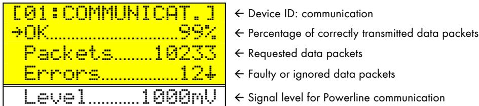
**Fig. 5.14:** Communication test
