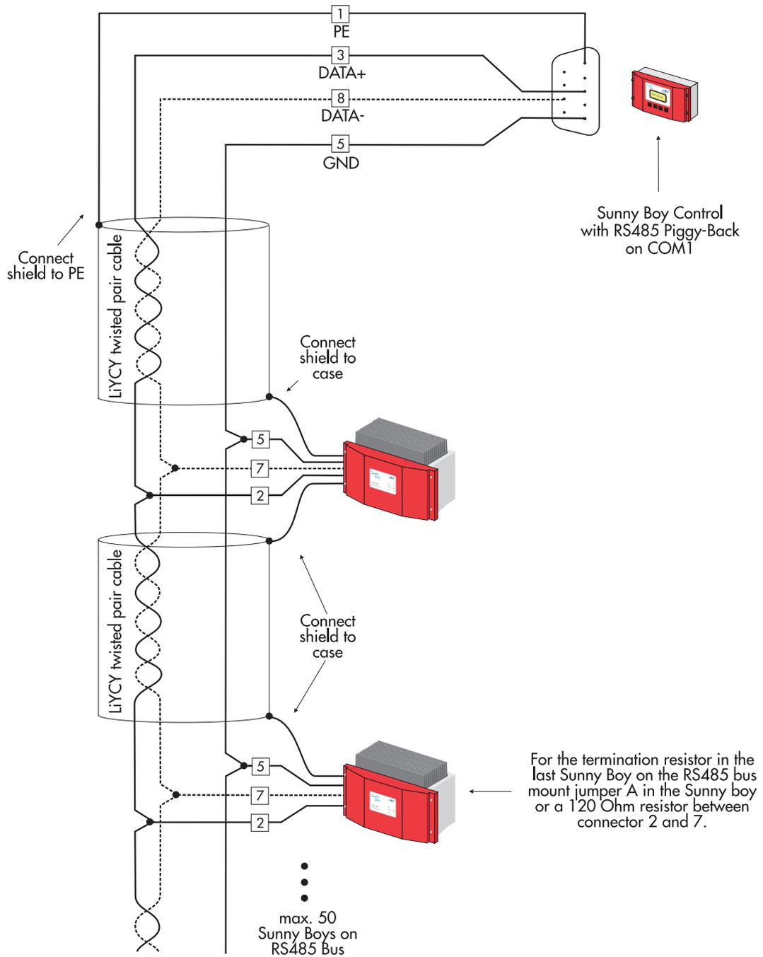
**Fig. 3.8:** RS485 connections between Sunny Boys and a Sunny Boy Control
