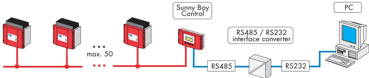
**Fig. 3.13:** RS485 connection to a PC
