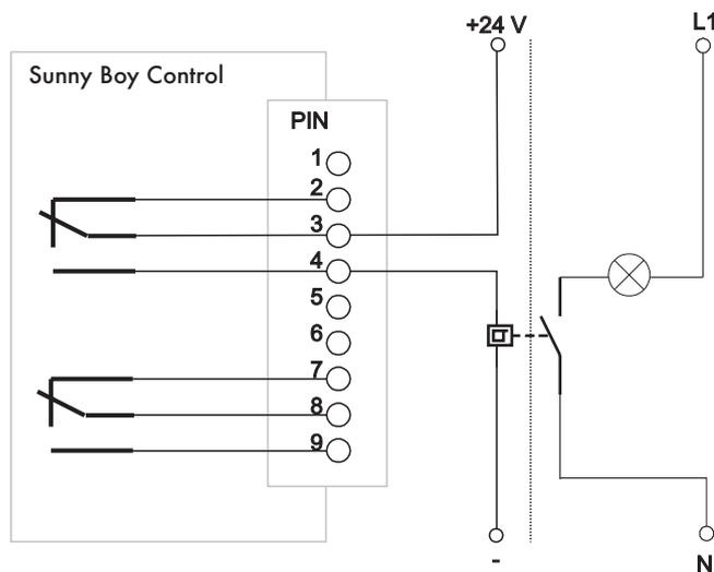
In this example, the "Default Switch" is set to "contact 2-1". If the external load is also to be switched in the event of a power failure, connect the relay to pin 2 and set the "Default Switch" to "contact 2-2".
