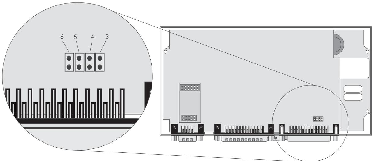
**Fig. 7.6:** Jumper configuration for measuring current
